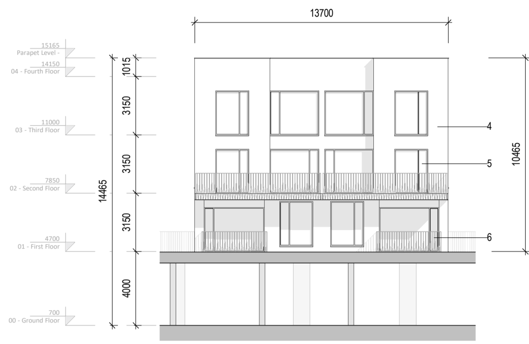
1 A2_Duplex South-West Elevation 1:200
